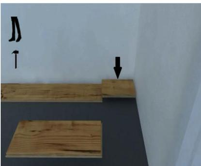
4. Continue connecting the first row until you reach the last full plank. Fit the last plank by rotating the tile 180° with the pattern side upward, place beside the row. Draw a line across the new plank with a pencil, score with a utility knife and snap off. Attach as described above.
